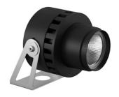
LED source included. Integrated electrical power supply 220-240V ON/OFF. Fixing bracket included. Equipped with a 1000 mm protruding section of neoprene cable and a kit with crimpable connectors and adhesive heat-shrinkable sleeves that guarantee the tightness of the connection. Optional IP68 connectors available. The metal nail for ground installation needs to be ordered separately. Optional accessories to regulate the light beam. Dimmable version available upon request.
