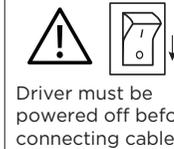
Before connecting the luminaire/LED module to the driver please make sure the driver is not powered but disconnected from the mains. The driver can only be powered when the luminaire/LED module is already connected. Disregarding this instruction might damage or even destroy the luminaire/LED module.
