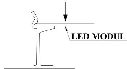
8.\*\*install the light source (see label on the luminaire)
