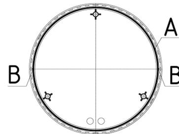
10. put the shade on and by angular rotate clockwise and tighten
