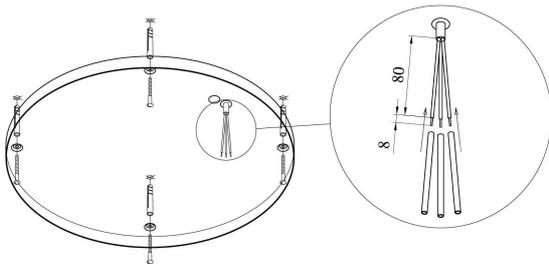
5. supply the input conductors with silicon sleeves
