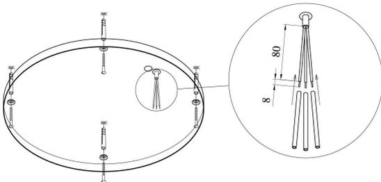
4. supply the input conductors with silicon sleeves
