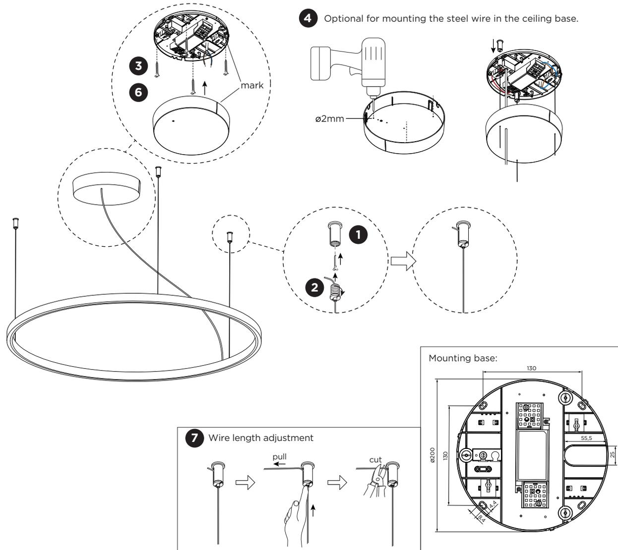
**4** Optional for mounting the steel wire in the ceiling base.
