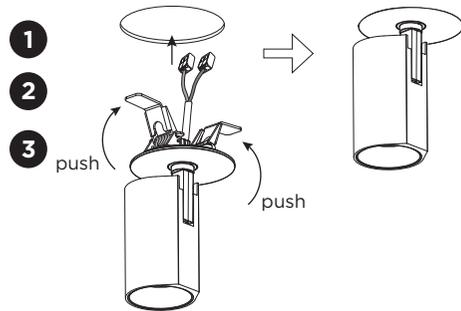
installation for 1.0 LED with blade springs
